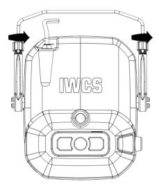
**2.** After loosening the nuts, you can adjust the earcups up and down according to your preference. Remember to tighten the nuts after making adjustments.
